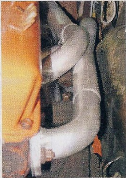
The steering column shaft actually goes through the header to the box.
