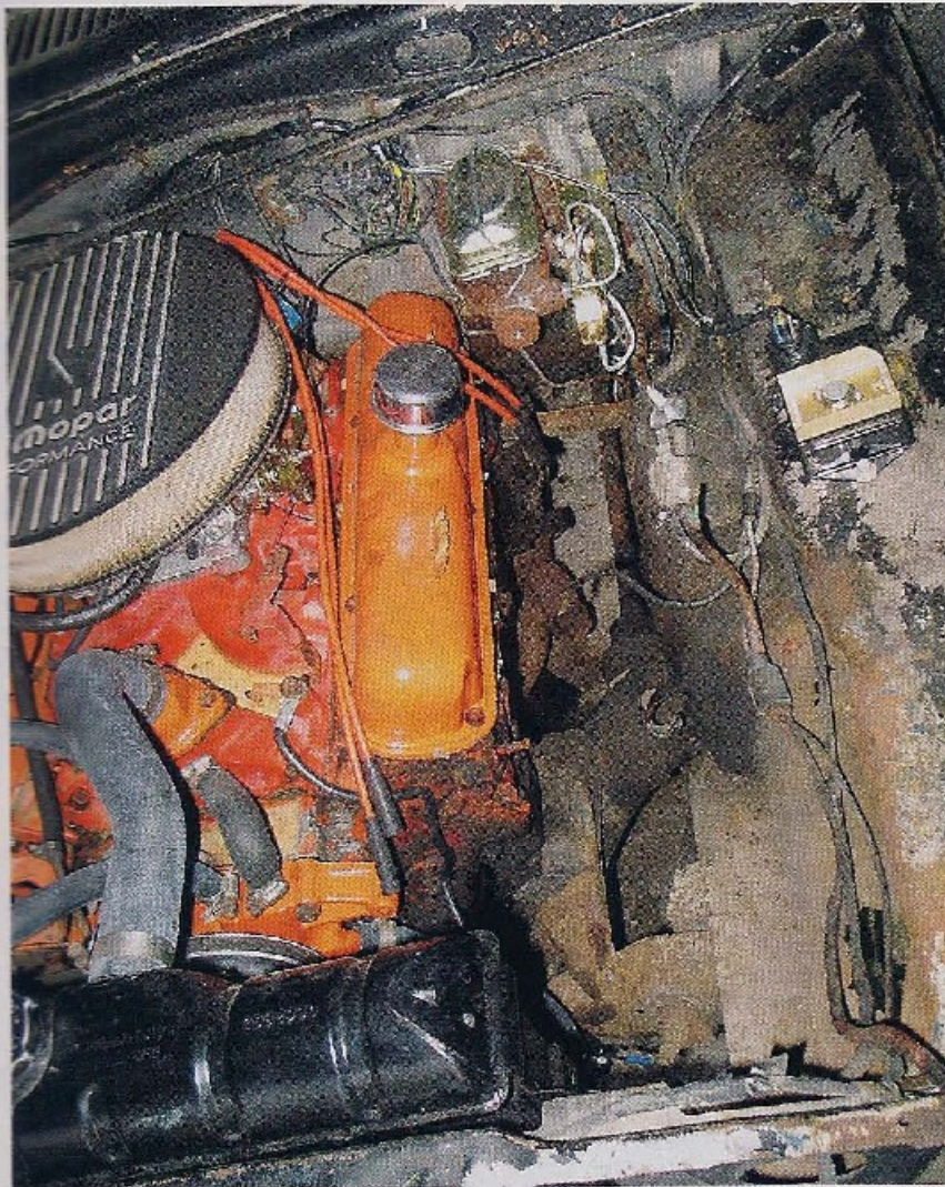
According to the instructions, items such as the steering column, starter, and steering linkage needed to be removed. We also found that removing the steering box made a lot more room and was worth the effort.
