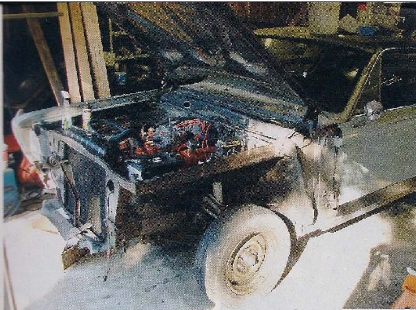
The car we checked fitment on is a '65 Barracuda that was ready for a restoration and has a V-8 with a four-speed transmission under the hood. You are going to need quite a bit of ground clearance to get the job done, so use the tallest jackstands you can find.
