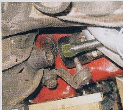
Much like the steering column shaft, the torsion bars also go through the headers. Before we re-installed the torsion bars, we cleaned them and gave them a fresh coating of grease.
