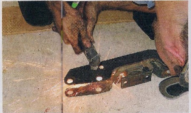
We broke out the trusty plasma cutter and modified the crossmember per the instructions. If you are unable to modify the crossmember yourself, tti can do it for you. ▶
