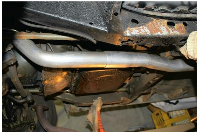
The intermediate pipe slid right onto the front exhaust pipe.
