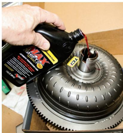
To prevent a dry start for our new TCI torque converter, we poured in a quart of TCI's Max Shift synthetic ATF. We coated the converter's snout with ATF to prevent possible damage to the T-Flite's new front seal.
