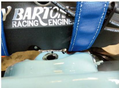
The Hemi was bolted back in place. Then, the trans was installed with its mount and crossmember to properly position the engine and trans. Here's the clearance we settled for with our Hemi valve cover. It's nearly  $\frac{1}{4}$  inch, which should be enough. If it hits while the engine is running and shaking, we'll put a rubber isolator in-between the gap.
