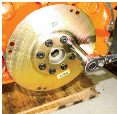
ARP crankshaft bolts (PN ARP-200-2905, Summit, \$33.95) were used to secure the TCI solid flexplate. The ARP fasteners received three steps of torque (40 to 60 to 85 ft-lb) in a crisscross torque sequence pattern.
