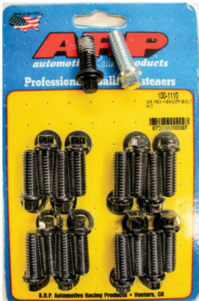
ARP header bolts (PN ARP-100-1110, Summit, \$20.99) were employed. These ultra high-quality bolts feature a 5/16-inch hex head making for easier access with a smaller wrench or socket. The supplied TTI header bolts (top right) have a larger 3/8-inch hex head. Notice the top left ARP header bolt has high-temp antiseize applied to its threads.
