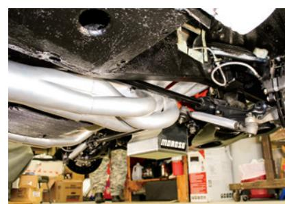
There's lots of clearance around all of the steering components and the PST 1.03-inch torsion bars we featured in a previous story, "Mopar Front Suspension Rehab: Get Handling With Stock Looks!" The prior dimpling of the number four header tube gave us a good ¼ inch of clearance of the T-bar.
