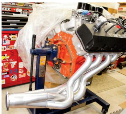
We're glad we straightened out the aforementioned clearance issues before implanting the Hemi into the engine bay. It would've been much more difficult and time consuming to work out the fitment of the headers to starter, block, engine mount, and dipstick inside the engine compartment.
