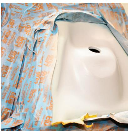
After clearance messaging the shock tower back by over a half inch, that area was sanded smooth and coated with Eastwood gray epoxy primer (PN 14149Z, Eastwood, \$22.99) for good rust protection. Online we found a spray can of B1 Blue to spot-in our handiwork. It's a shade darker than the powder blue, but most folks won't notice.
