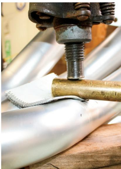
The headers easily bolted in without the torsion bars in place. Only the left side requires the engine to be raised an inch. Once installed, the L/S side header touched the Borgeson quick-ratio power steering box. The R/S header was rubbing the torsion bar. Shown here, we're dimpling the R/S header using a hydraulic press, piece of leather, 1-inch brass drift and a few blocks of wood while trying not to scratch the ceramic coating on the TTI headers.
