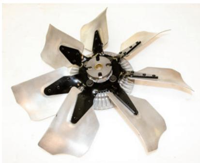
We discovered Hayden makes a quality thermal clutch fan (PN HDA-2765, Summit, \$41.99) that's the same depth (2 5/8 inches) as the original unit. Here, we bolted it to the '65 aluminum-bladed fan for a cool period look. The '66-and-later fans came equipped with heavier steel blades. The lighter aluminum blades should save us a few horsepower.
