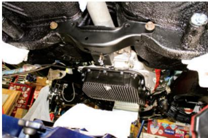
To be sure of proper engine position, we bolted up our A&A trans with the Schumacher mount and stock cross-member. Now we could be exactly sure of where the valve cover was hitting the shock tower. At this point all other clearance checks looked good and the car's original '65 cable-shift, slippyoke Torque-Flite was back in its original location.
