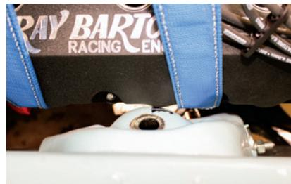
Here's where the taller and wider Ray Barton Racing Engines valve covers were hitting the shock tower. If we used stock valve covers there wouldn't be any clearance issues, but we must use these fat valve covers to clear the Ray Barton rocker arm system. The Barton rocker setup gives you superior valve-train geometry for more power and rpm.
