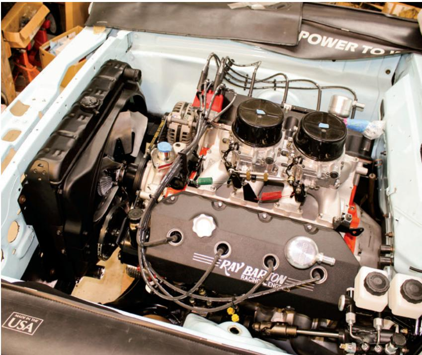
We're so happy our Street Hemi is finally sitting pretty in its home. Next, we'll attend to the wiring, plumb the cooling, fuel and exhaust systems. We also have to measure for a QA1 carbon-fiber driveshaft. Then, we can fill it with fluids, bleed the Wilwood brake system, and finally fire up this bad-to-the-bone, pump-gas, 825hp Barton Street Hemi. We can't wait to hear it through the TTI 3-inch exhaust!
