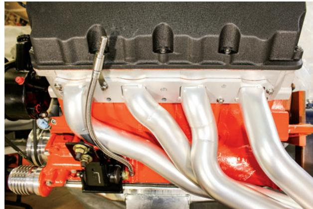
Fitment with the Milodon dipstick worked best when mounted and routed as seen here. Routing/mounting it any differently made pulling and putting in the dipstick very difficult, if not impossible.
