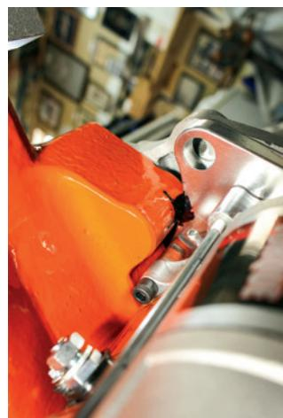
The newer Mopar Gen II Hemi blocks are beefier than the original factory castings. To line up the starter bolt-holes, we'd need to clearance grind the block or starter. TTI Exhaust recommends use of this clock-able Powermaster XS Torque starter (PN PWM-9523, Summit, \$308.99) for fitment with their headers.
