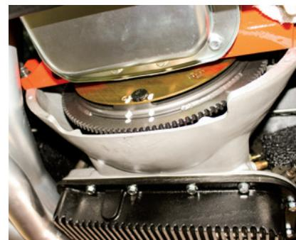
The previously mentioned white paint marks came in handy to easily line up the converter to flexplate bolts into their respective holes. Here, we also used ARP bolts (ARP-240-7302, Summit, \$10.99) to handle the Hemi's torque for no fear of fastener failure
