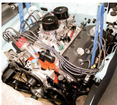
The conversion engine mounts from Schumacher Creative Industries helped us ease the massive Elephant into this sitting-pretty position. The Coronet's original V-8 K-member was powder-coated in a previous story while using PST's Polygraphite front end kit and suspension components when we rebuilt the front end.
